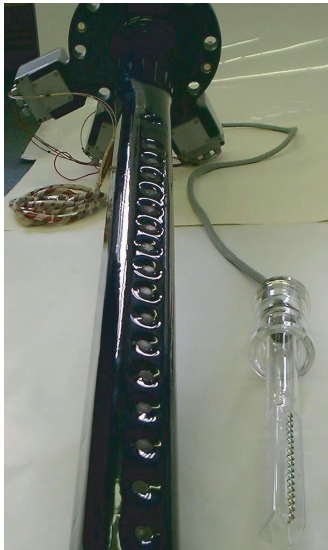
Figure 10. Glass-lined steel beaver tail baffle and glass baffle fitted with linear tomography array.
